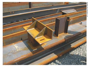
Supporting connections for the precast panels were welded to columns in the fabricator's shop, greatly reducing field welding requirements.
